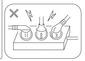
★ It must be used on the plug more than 120V/25A, 220V/15A individually.
