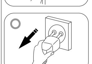
★ In case of pulling power plug, the hand must grasp the plug. Pulling plug in same method as pulling power wire with hand is prohibited.
