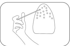
★ Vapour hole on press iron baseplate may be blocked by foreign matters, which requires cleaning by prod often.
